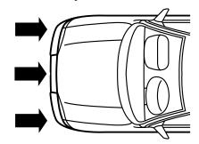
cause activation. Air bags are designed to inflate in frontal and near-frontal collisions, not rollover, side-impact, or rear-impacts.
